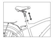
To enable comfortable, fatigue-free and safe riding, the saddle and handlebar height should be adjusted to the body size of the rider.
