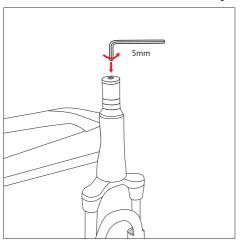
1. Remove the upper screw of the fork steerer tube.
