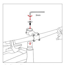
3. Install the handlebar and stem as shown in the above image, making sure none of the cables are twisted or too tight (you may have the handlebar twisted). Put the top cap with screw into the stem and fasten the screw (or the ball-bearings could get damaged) to secure the stem down onto the headset.
