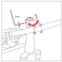
4. Align the handlebar vertically with the wheel (you may need to loosen the screw from step 3 to make small adjustments) and tighten the bolts on both sides of the stem.
