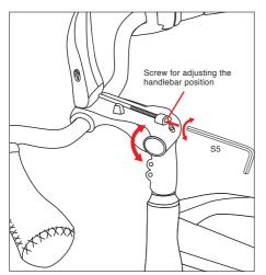
3. Move the handlebar up or down to adjust to the desired angle, then tighten the rear-facing screw at the top of the stem to lock the handlebar in place.
