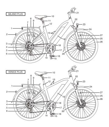
1 Rear Light 2 Rear Reflector 3 Motor 4 Freewheel 5 Rear Derailleur Protector 6 Rear Derailleur 7 Rear Disc Brake 8 Carrier 9 Bungee Cord 10 Saddle 11 Suspension Seatpost 12 Saddle Quick Release 13 Water Bottle Bolt 14 Chain 15 Kickstand 16 Pedal 17 Crankset 18 Controller 19 Battery 20 Front Disc Brake 21 Adjustable Stem 22 Frame Number 23 Front Light 24 Mudguard 25 Front Fork 26 Tyre 27 Wheel Reflector (reflectors may differ by country)
