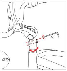
Align the handlebar to be perpendicular to the wheel, then insert and tighten the two side-facing screws as shown below.
