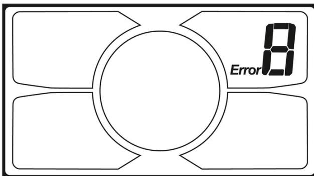
\* The display cannot return to normal status until the problem is solved; the E-bike's electric components will not operate if there is an error in the system. However, the bike can still be operated conventionally (without electric assistance).
