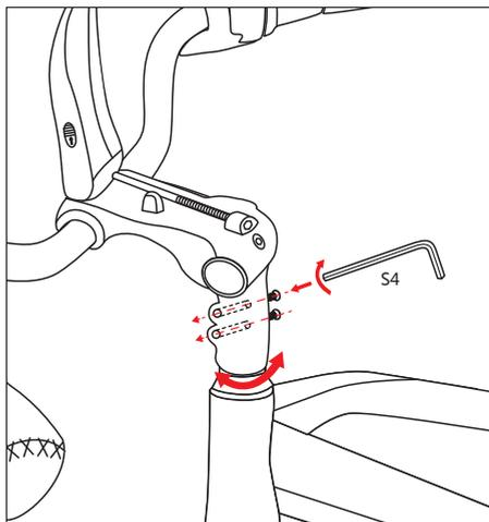
2. Align the handlebar to be perpendicular to the wheel, then insert and tighten the two side-facing screws as shown below.
