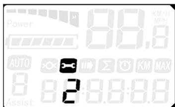
※The display cannot return to normal status until the problem is solved; the E-bike’s electric components will not function if there is an error in the system. However, the bike can still be operated conventionally (without pedal assistance).
