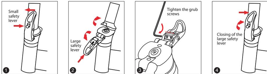
1. Press the small safety lever at the interlock upwards, to open the folding mechanism.
